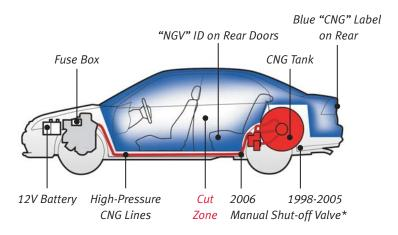
\*On driver's side. Turn one-quarter turn clockwise to shut off CNG.
